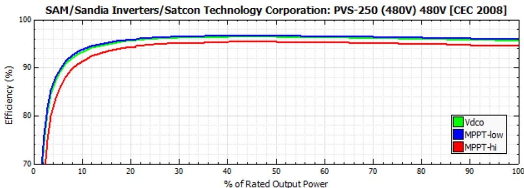
Figure 1. Inverter efficiency curve<sup>8</sup>
