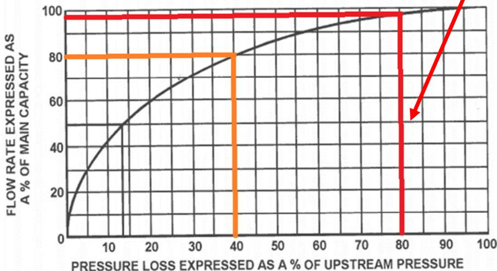
**Figure 38. Relation between flow rate and pressure loss for a main operated at high pressure.**<sup>19</sup>
