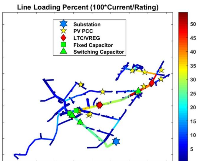
**Figure XI. 18.** Rural Feeder: Line Loading With Maximum Solar PV Output Under Minimum Load Conditions
