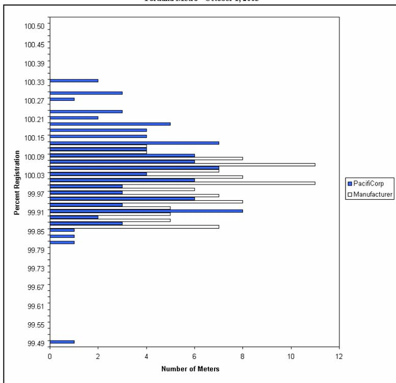
GE I-70-S Single Phase - Full Load Test - By Meter
