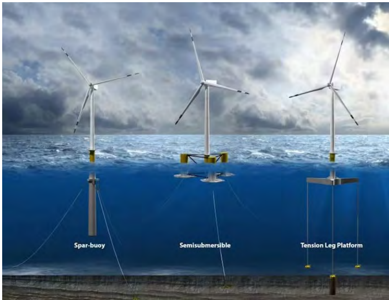
Three of the common types of floating wind turbine platform. Source: NREL
