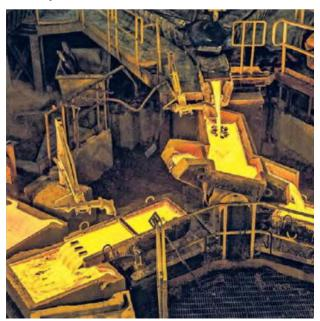
Left: Molten copper pours into ceramic molds to form plates in Peru.
