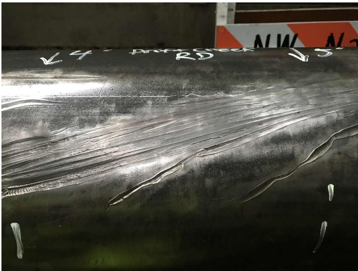
**Figure #3 Metal loss caused by cable dragging along pipe**
