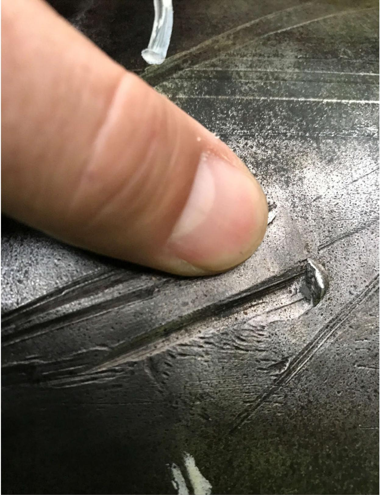
**Figure #4 Metal displacement caused by cable dragging along pipe**
