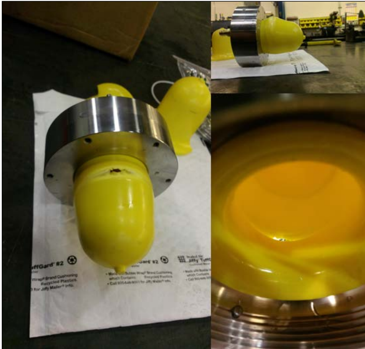
Figure 8-3. Ductile failure in un-notched UTV
