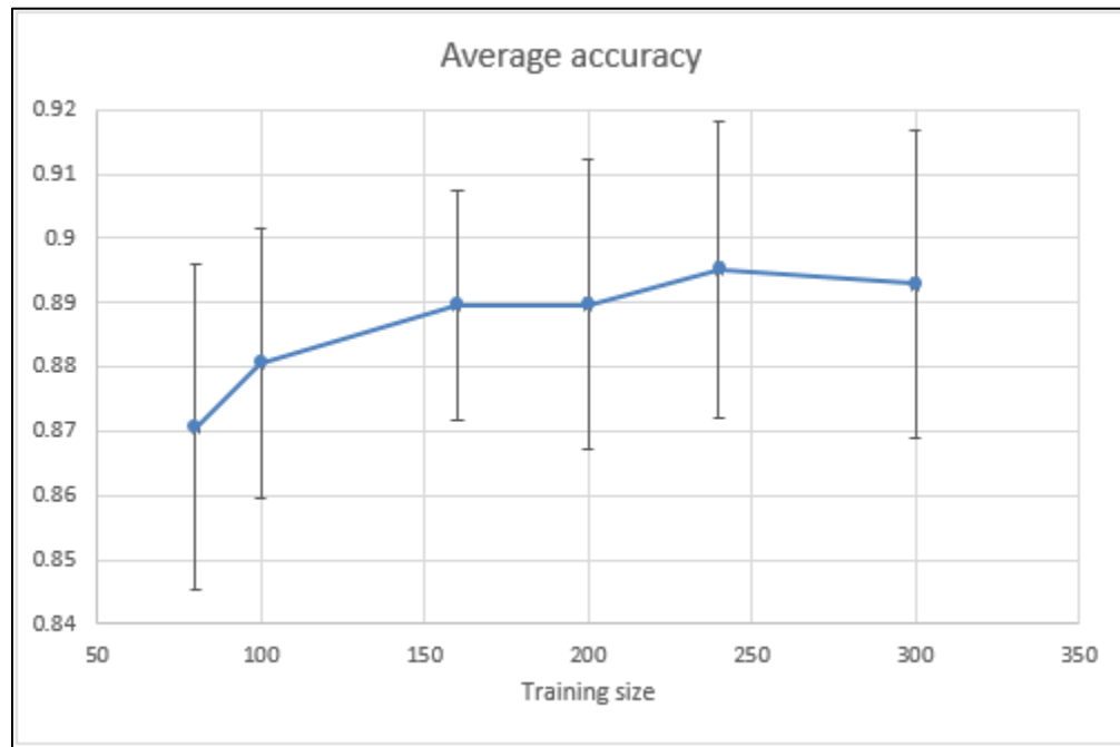
Figure 6-4. Average accuracy vs. training data size with simulated feature data
