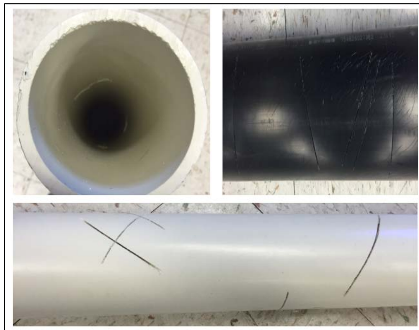
Figure 5-13. The linear cracks in the spacemen
