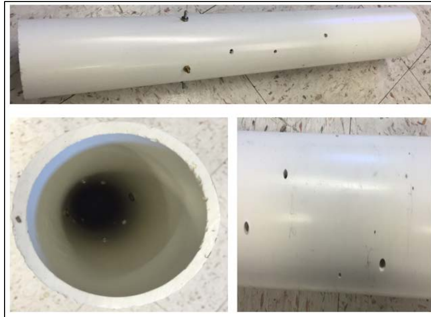
Figure 5-12: The holes that have been introduced as defects
