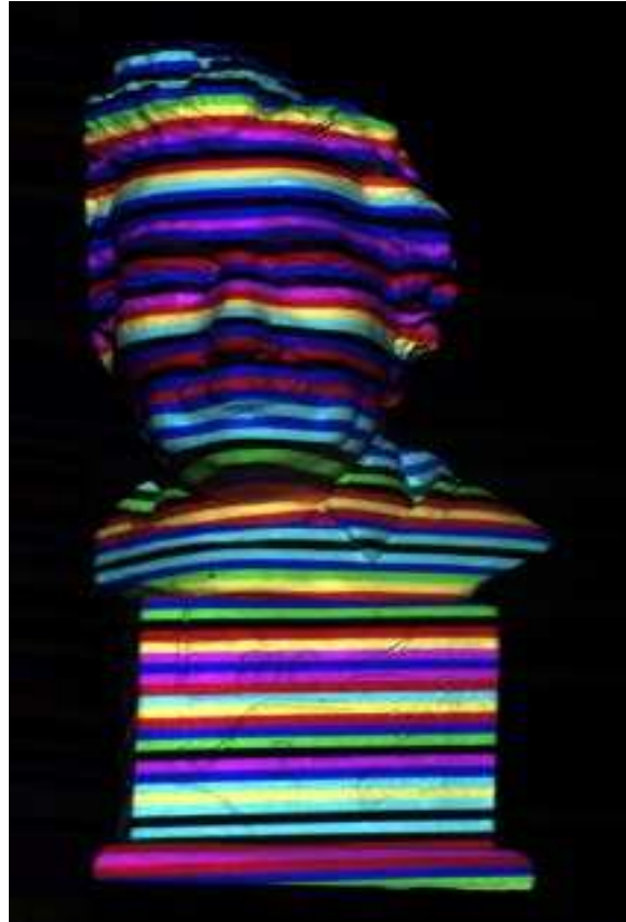
Figure 5-1. Example of a structured light pattern projected onto an object [30]
