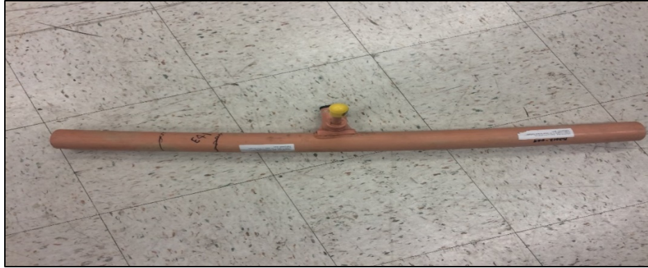
Figure 5-14. Pipe with a small diameter (1.85 inches) and damage section
