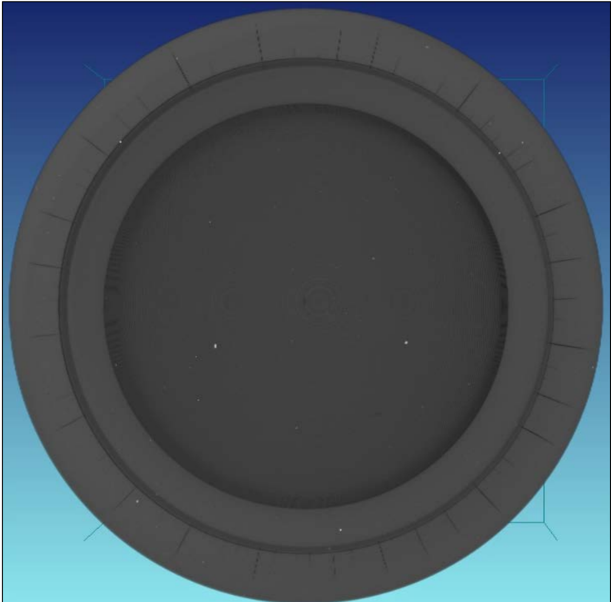
Figure 8-12. Computerized X-Ray Tomography section through UTV showing multiple damage fronts propagating radially outwards from the notch tip
