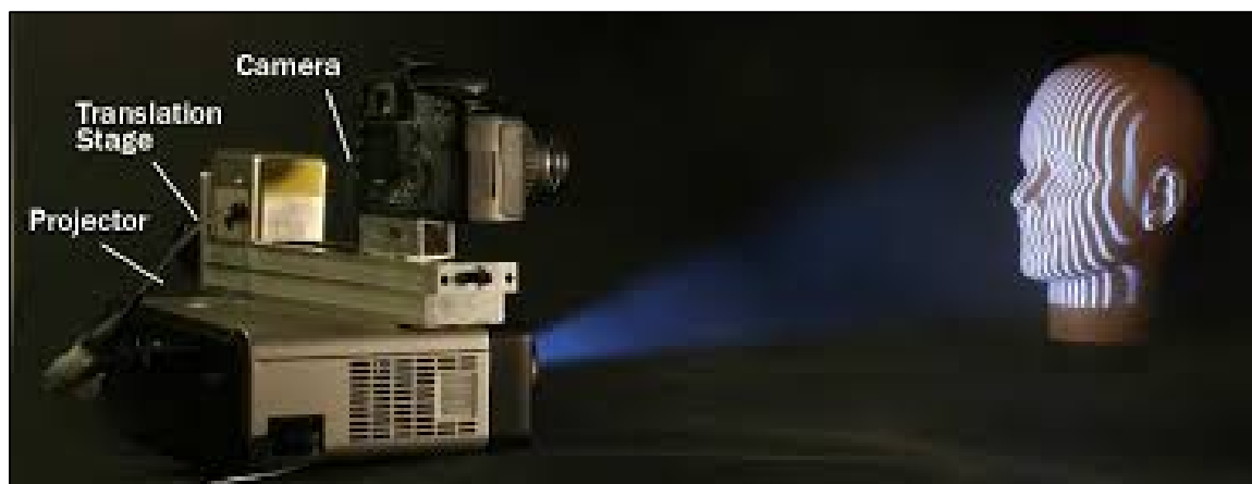
Figure 5-42. Structured light with a projector used to generate the [45]
