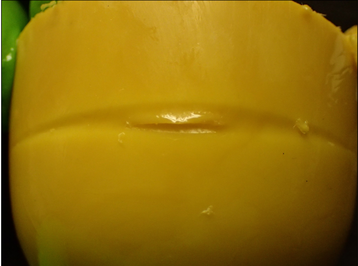
Figure 8-4. Ductile failure initiated at the stress riser notch
