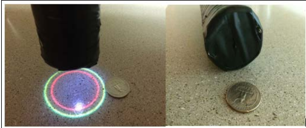
Figure 5-54. a) the projection on the smooth surface. b) the prototype with blocked edges
