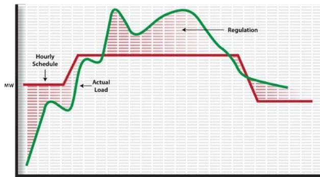
**Figure 3. Reduced Regulation Requirements With Subhourly Dispatch<sup>46</sup>**
