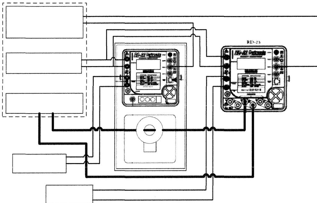
Figure 1 – Equipment setup to test transport standard
